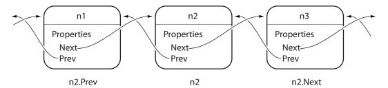
To add a new node to the list, it is necessary to disconnect the existing nodes in the list, insert the new node, and reconnect the nodes appropriately. Here are the basic steps:
