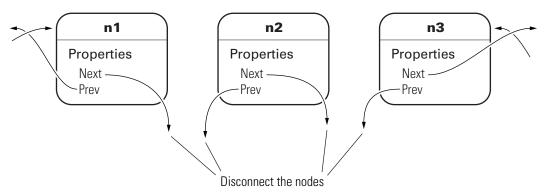
removeNode removes n2 from the list and repairs the list with the following steps:
