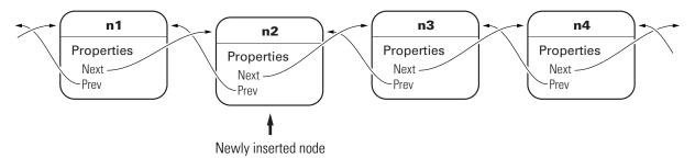
The details of how methods perform these steps are encapsulated in the class design. Each node object contains the functionality to insert itself into or remove itself from the list.
